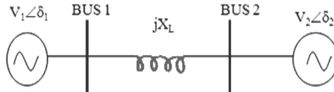
**Figure 1: Simplified Model of Power Transmission System**
