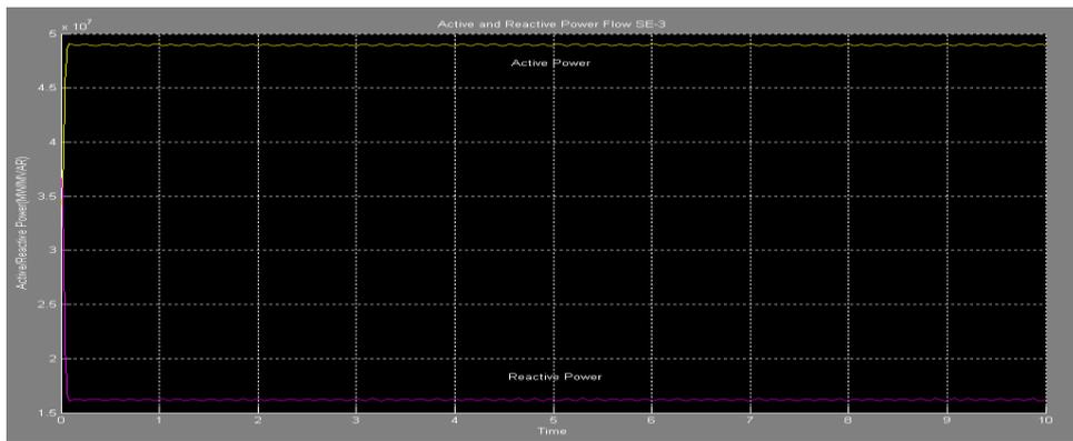
**Figure 10: Active and Reactive Power Flow at Sending End of Transmission Line Compensated by SVC Installed at Load End**
