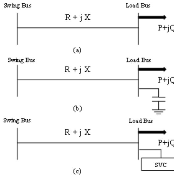
**Figure 5: (a) Transmission Line without Compensation (b) Transmission Line Compensated by HT Shunt Capacitor Bank (c) Transmission Line Compensated by SVC**
