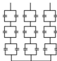
Figure 3: 33 KV 5.43 MVAR HT Shunt Capacitor Bank with Three Series Group
