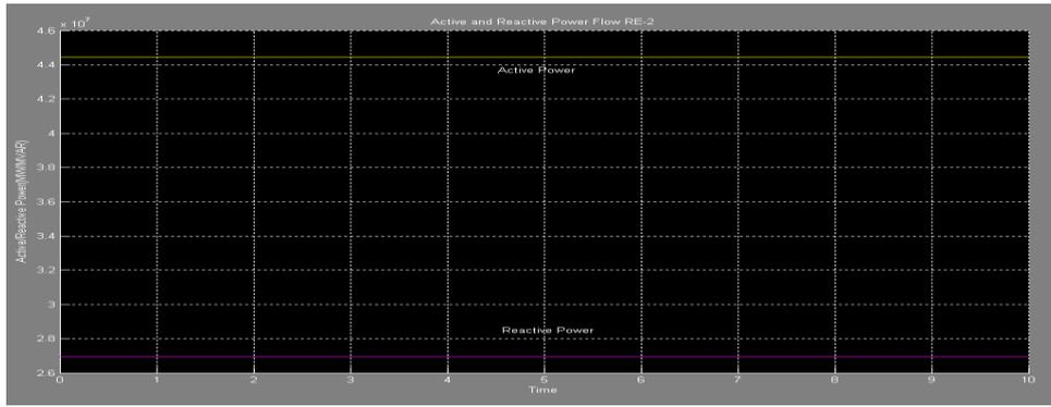
**Figure 9: Active and Reactive Power Flow at Receiving End of Transmission Line Compensated by HT Shunt Capacitor Banks**
