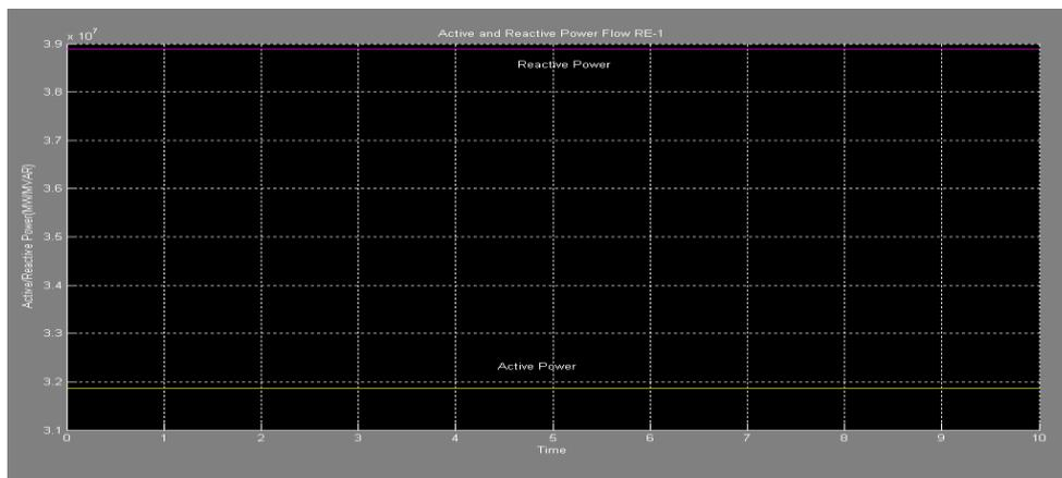
**Figure 7: Active and Reactive Power Flow at Receiving End of Uncompensated Transmission Line**
