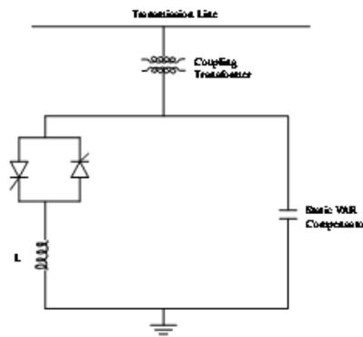
**Figure 4: SVC Connected to Transmission Line**
