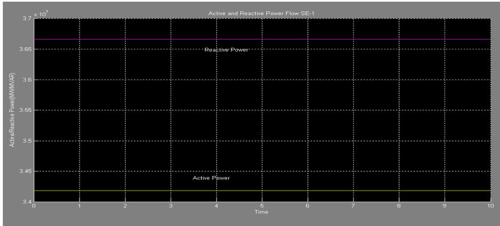
**Figure 6: Active and Reactive Power Flow at Sending End of Uncompensated Transmission Line**
