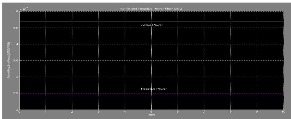
**Figure 8: Active and Reactive Power Flow at Sending End of Transmission Line Compensated by HT Shunt Capacitor Banks**
