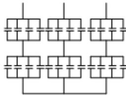
Figure 2: 33 KV 5.43 MVAR HT Shunt Capacitor Bank with Two Series Group
